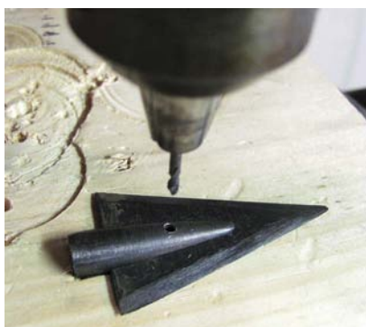
(below) Author's method of drilling the head for the rivet.
