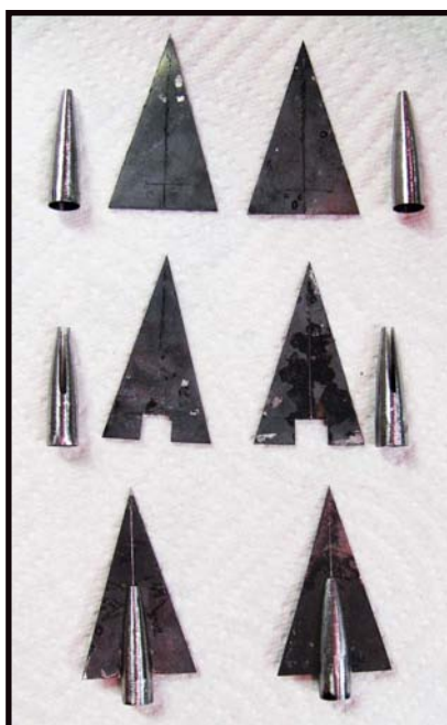
Steps of assembly. Top row shows the ferrules and the blades after grinding. The center row identifies the ferrules with a slot cut in them to accept blades. The blades are then notched to accept the ferrules. And, finally, the assembled parts ready to be drilled for rivets.
