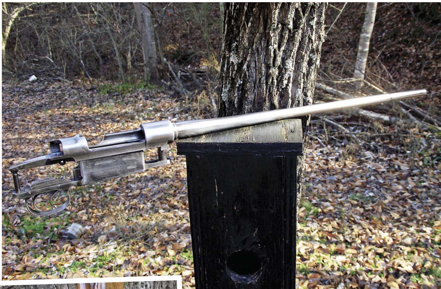
(above) This is a polished Mauser barrel and action ready to be rust-blued.
